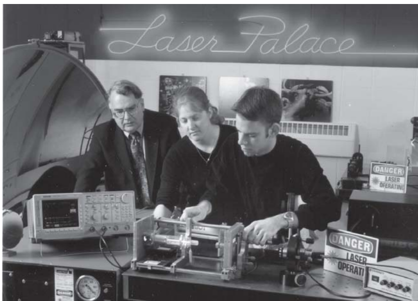
Working in the Laser Palace, Dr. Brandenberger and students examine the spectral lineshape of an open-frame, narrow-bore, helium-neon laser.
