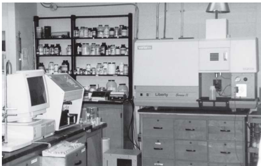
Furman's well-equipped laboratories include a liquid chromatograph, left, and an inductively coupled plasma-atomic emission spectrometer, center.
